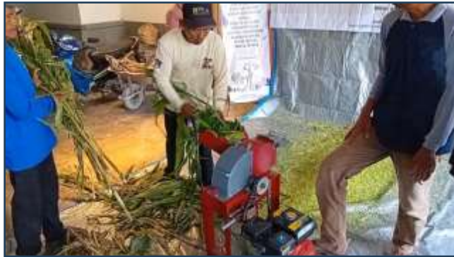
Gambar 4. Proses coper bahan silase
